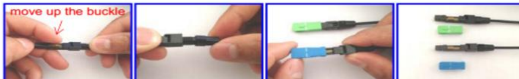
9. Keeping the fiber micro-bent, and move up the buckle to block the fiber
